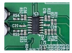
On top (parallel) on C19 and C14 a 10m resistor m needs to be placed.
